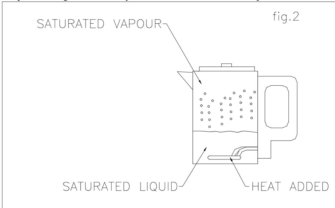
Heat is added to the liquid (which in this case is water) causing its temperature to rise until it reaches its boiling point. When the liquid reaches its boiling point it begins to change into steam.
