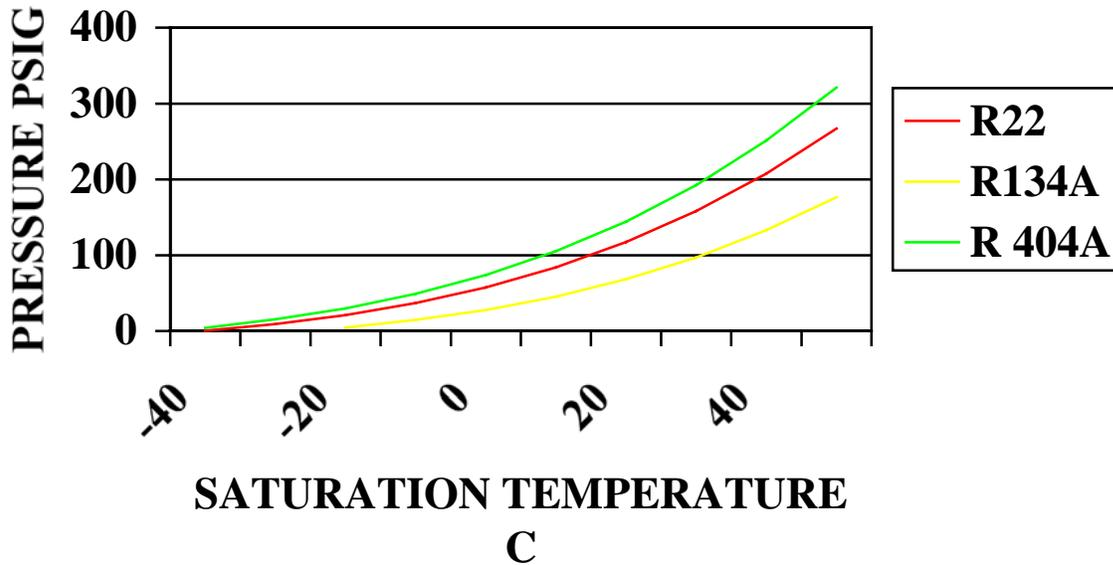
The boiling point of any single component refrigerant will change according to the pressure which is acting upon it. As the pressure in the refrigerant increases, the boiling point also increases and conversely as the pressure falls so does the boiling point.
