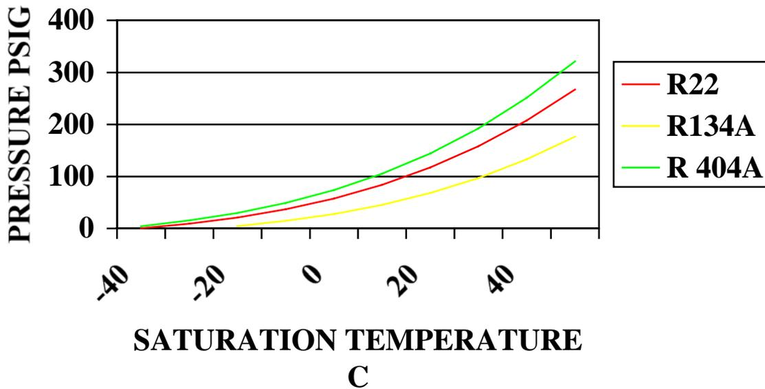
The boiling point of any single component refrigerant will change according to the pressure which is acting upon it. As the pressure in the refrigerant increases, the boiling point also increases and conversely as the pressure falls so does the boiling point.
