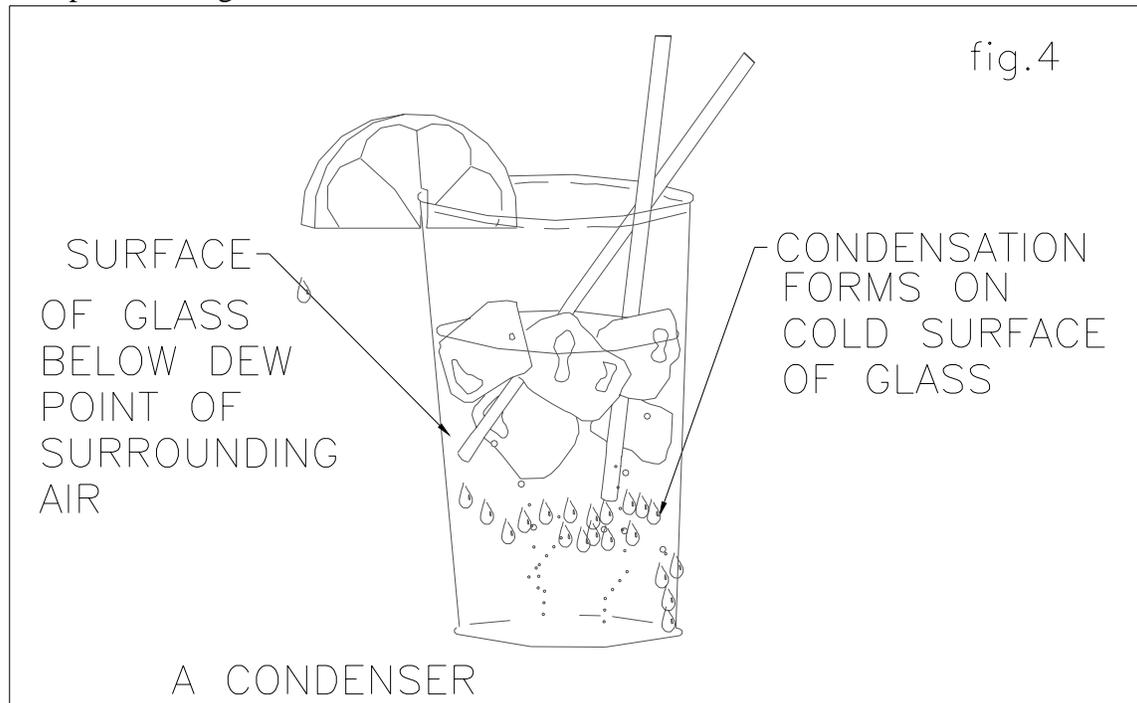
You will all have seen how condensation forms on the surface of a cold glass in the Summer. This is caused by the glass absorbing the latent heat from the water vapour contained in the air surrounding the glass. This causes the vapour to return to a liquid state.
