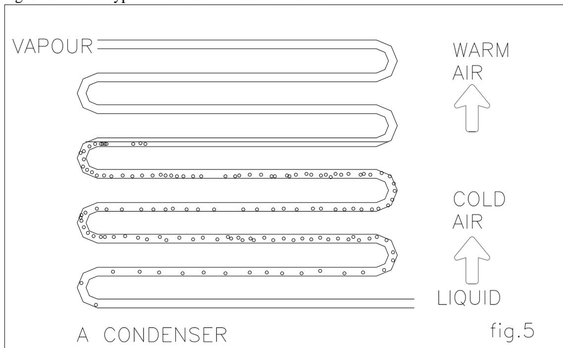
Note the similarity to the evaporator which we saw in fig.3. This time vapour at high temperatures is passed inside the tubes. Cold air is blown across the coils to remove the latent heat and the refrigerant turns into a liquid.
