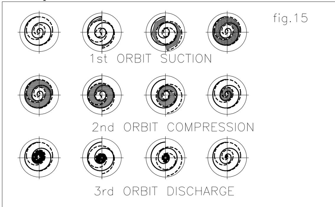
The scroll compressor is quite a new design of compressor. The compressor has two scrolls ,one rotating and one fixed. The scrolls move relative to each other to create pockets into which refrigerant is drawn and compressed Fig. 15 shows the way that the scroll compressor operates.
