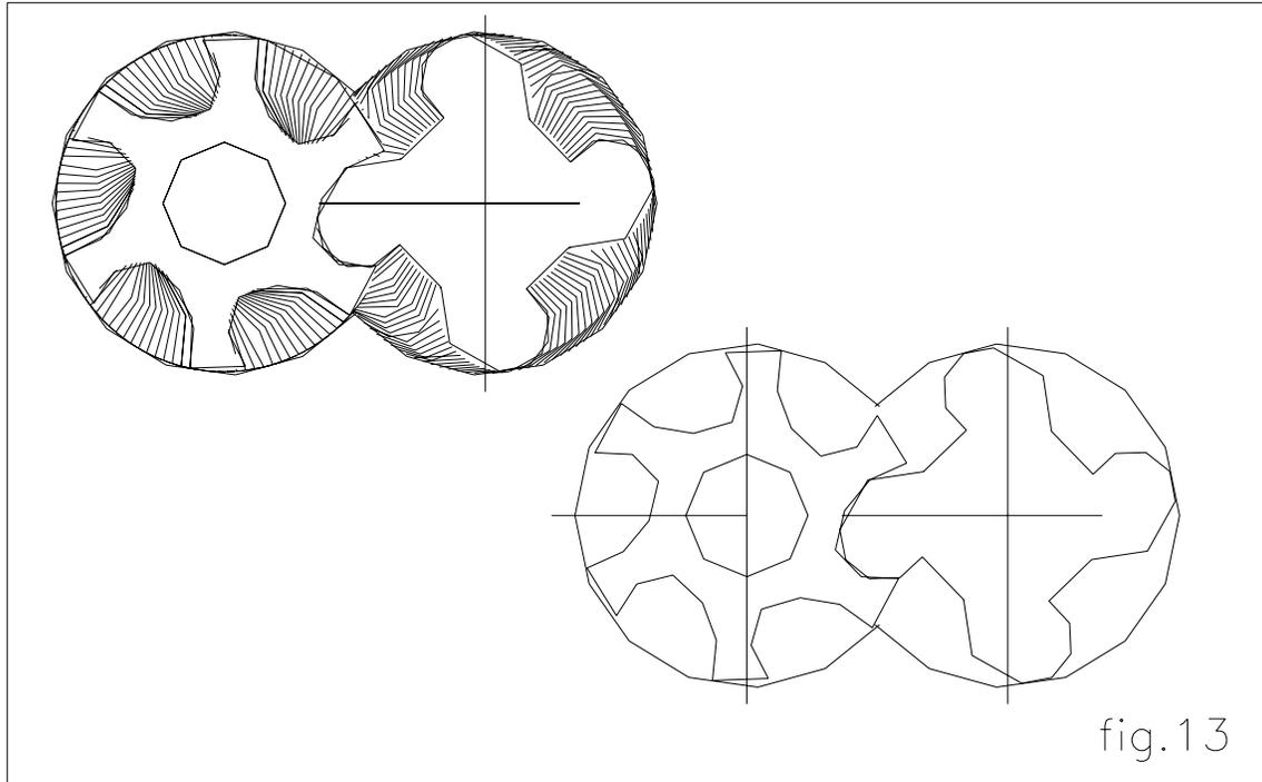
The twinscrew compressor has two main rotors. One rotor is fitted with six paths whilst the other is fitted with 4 lobes. This is shown on fig.13. As the compressor rotates the refrigerant gas is pushed forward by the two rotors in a similar way that toothpaste is squeezed out of a tube when the bottom is pressed. Again these compressors are designed so that the following compression has already started before the first one has finished ,giving a continuous,non pulsating output.
