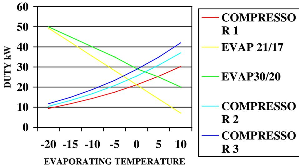
As previously discussed an evaporator is continuously boiling off liquid refrigerant which is entering the coil through the expansion valve. The quantity of refrigerant that it is capable of evaporating is determined by the energy levels of the air entering the coil and the ability of the compressor to remove the evaporated refrigerant.
