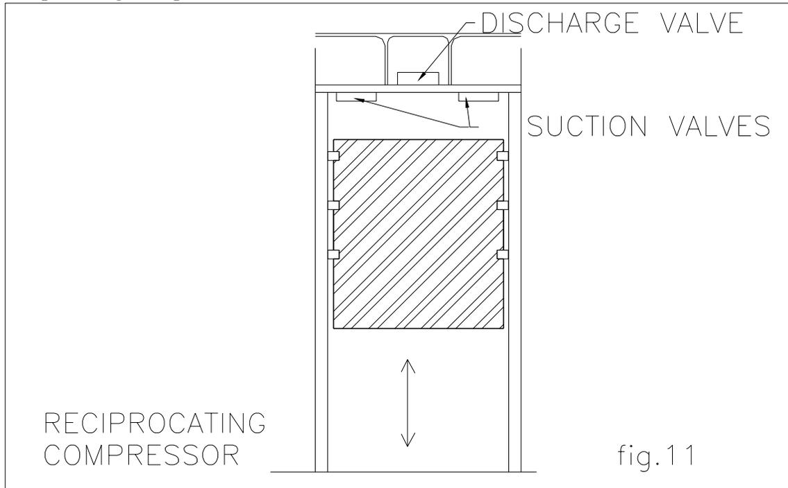
In reciprocating compressors the refrigerant is compressed by one or more pistons drawing refrigerant into a cylinder and then pushing it out again into a much smaller volume. The compression given by this type of compressor is in the form of pulses of high pressure refrigerant. The number of pulses is determined by the number of cylinders which operate for a single revolution of the crankshaft and the speed at which the crankshaft turns.
