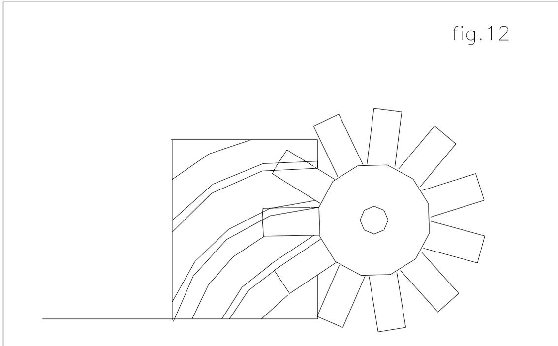
The monoscrew compressor is constructed with a single screw which meshes with 2 gate rotors. As the main rotor turns, the gas is pushed along the grooves in the screw by the blades on the gate rotors and is compressed until the end of the screw passes the outlet from the compressor allowing the compressed gas to be discharged into the system. As the rotors are placed to follow each other, the compression from this type of compressor is continuous. fig.12 shows this.
