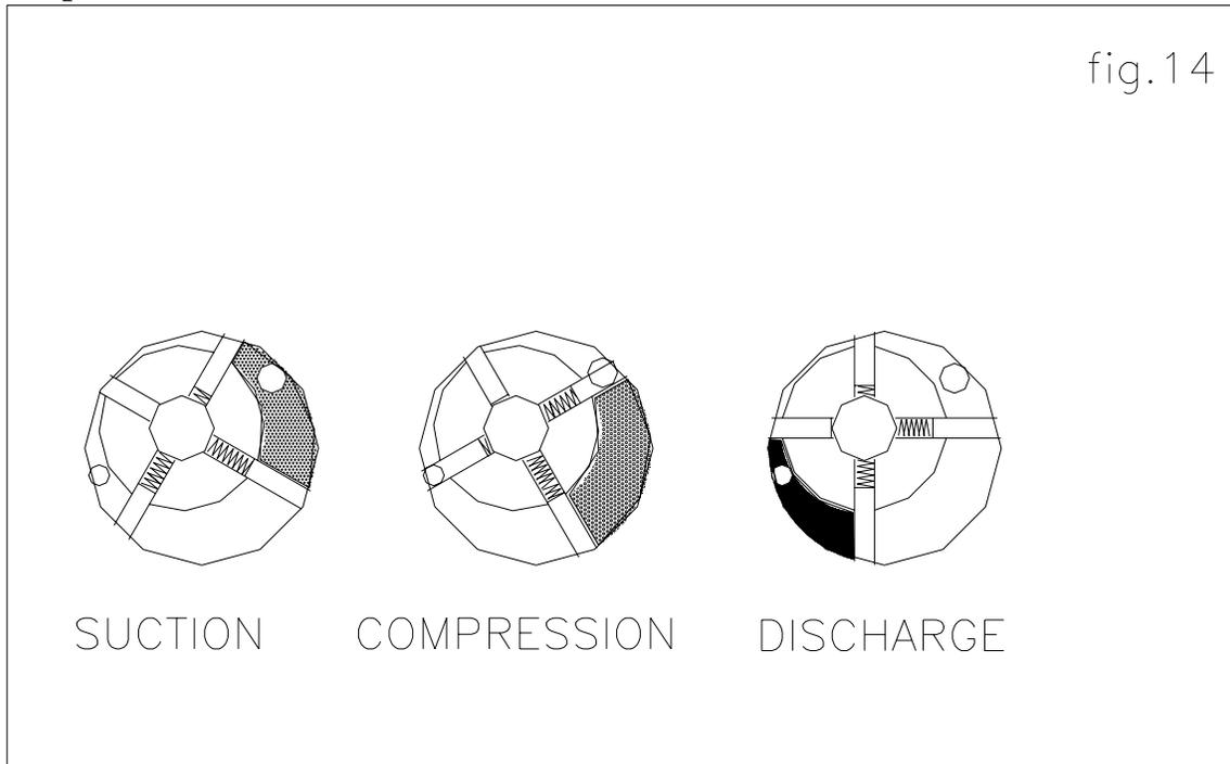
Rotary compressors are used on very small equipment ,usually in air conditioning. The compressor consists of a rotor with a number of sprung loaded vanes. This rotor runs eccentricly in a ring which causes the refrigerant to be compressed.Fig.14 shows a typical arrangement. The advantage of these compressors is the lack of moving parts which can wear out. These compressors are generally supplied as hermetic type only.
