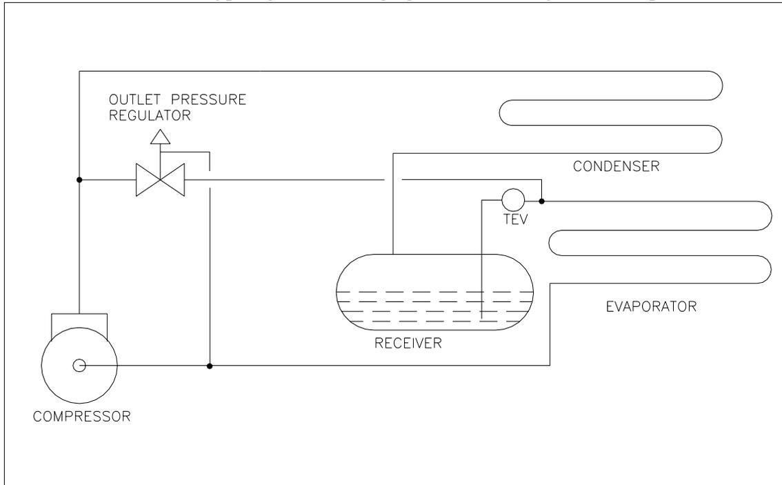
This does two things, firstly it put a quantity of heat into the coil which will assist in boiling off the liquid refrigerant present. The second thing that happens is that a quantity of vapour from the compressor forms a part of the total vapour drawn back to the compressor and therefore has the effect of reducing the mass flow of refrigerant being circulated. This type is most frequently used where the evaporator is close to the compressor or condenser.
