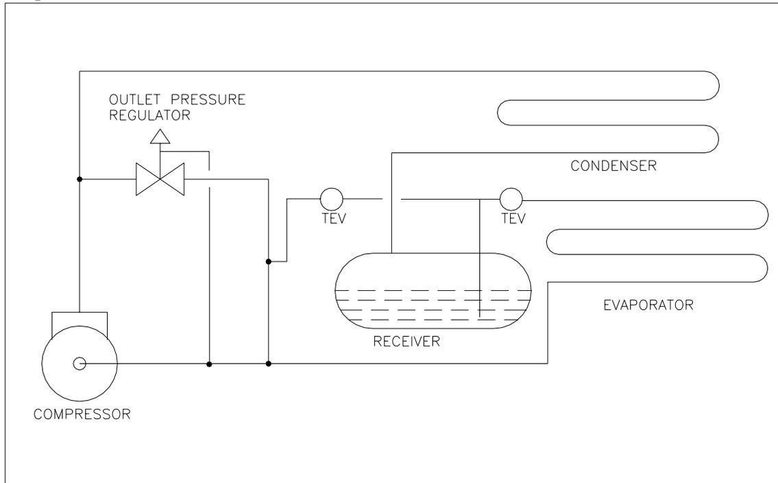
It does not introduce any heat into the evaporator. With this type of control it is usual for a liquid injection valve to be fitted which will cool the discharge gas before it is returned to the compressor.
