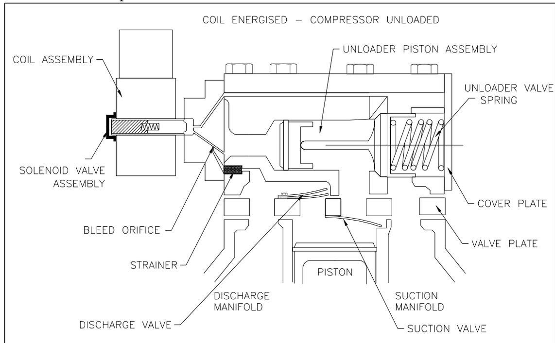
This lets gas from the chamber behind the unloader piston to bleed to suction pressure. The spring pressure is now sufficiently high to move the piston against the pressure in the chamber behind the piston which lets the valve close. Once the valve has closed no gas can reach the suction side of the valve plate and no compression takes place
