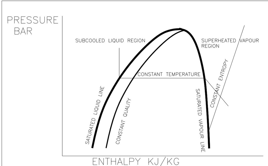
Here we see a similar chart to the original but containing further information. It represents a single component refrigerant such as R22 and it can be seen that lines of constant temperature correspond with lines of constant pressure. That means that there is only one saturation temperature for a given pressure irrespective of the state of the fluid.
