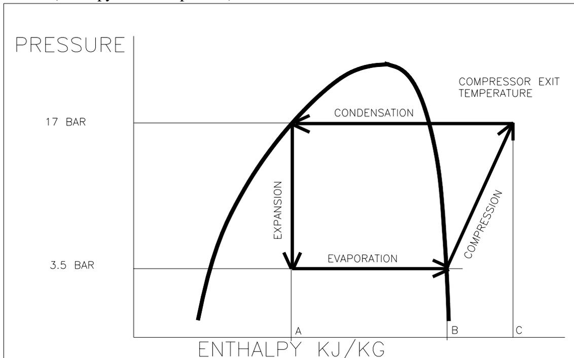
This chart shows the final part of the cycle. Heat is removed from the refrigerant until the enthalpy is reduced to the level at A where the cycle begins again.
