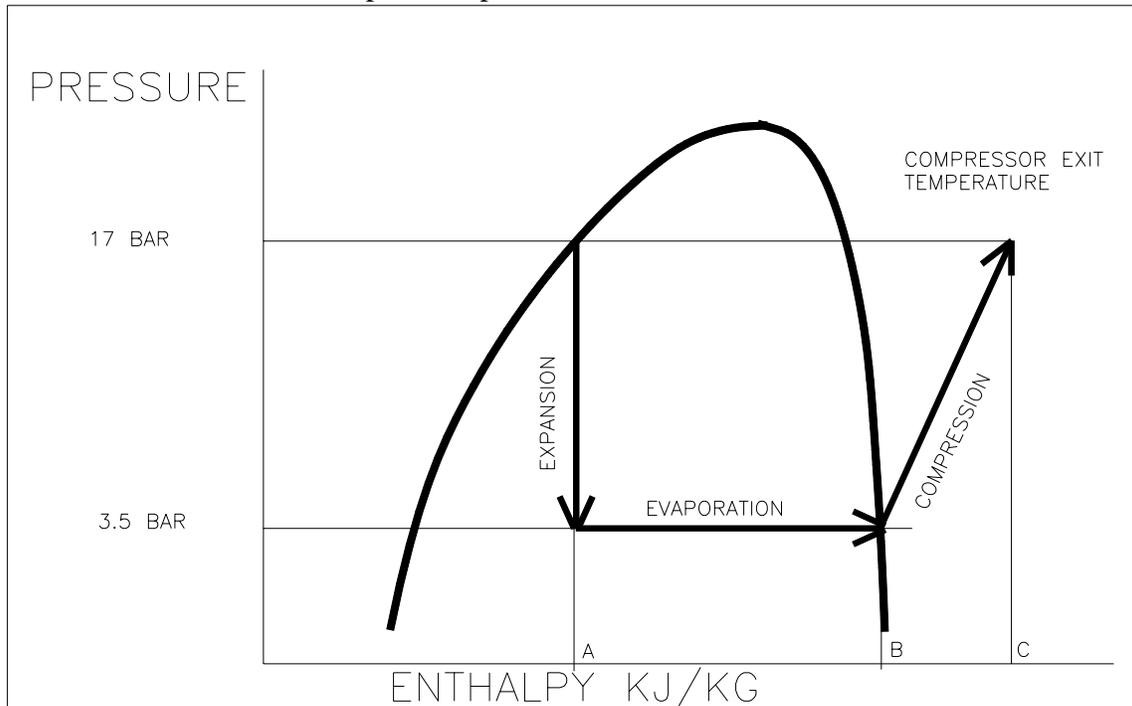
The act of compression requires energy to be added in the form of mechanical work. This is transformed into heat and the compression process follows the line of constant entropy. The point where it reaches the condensing pressure defines its temperature and its energy content (enthalpy is now at point C).
