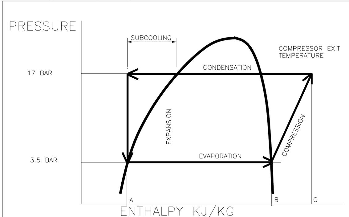
You will note that the expansion phase has moved to the left of the saturation line and the entering liquid enthalpy has reduced.
