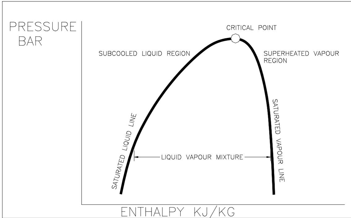
This diagram shows a simplified pressure/ enthalpy chart for a non specified refrigerant. The area contained within the envelope is for a liquid vapour mixture. The region to the left of the envelope represents liquid in a subcooled condition. The region to the right of the envelope represents vapour in a superheated condition.
