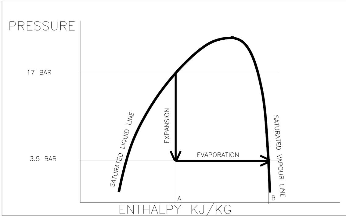
On this chart we have added the expansion process. The line moves horizontally to the right until it reaches the saturated vapour line. The enthalpy has increased from A to B. This means that energy has been absorbed by the refrigerant and this energy has been removed from the air stream.
