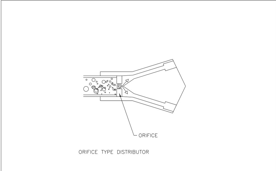
Orifice type distributors have a disc with a circular hole (or orifice) which determines the flow capacity. All the larger coils use this type of distributor.
