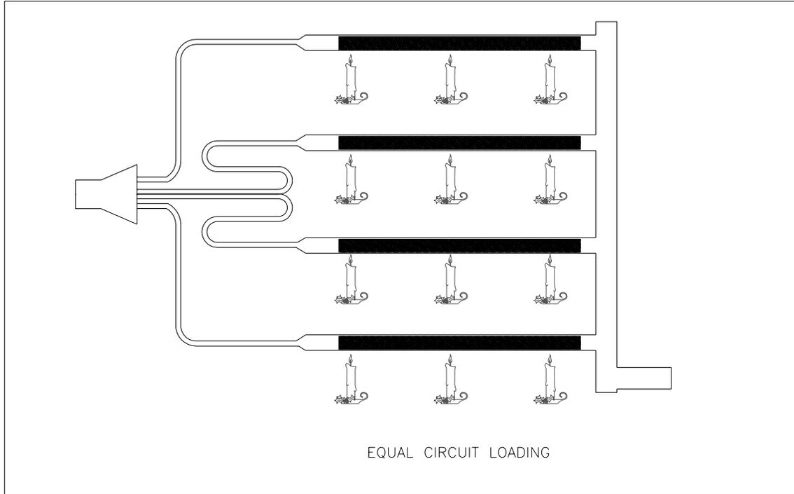
This diagram shows a properly circuited coil. Each of the circuits has the same amount of heat applied and the liquid finishes boiling off at the same position.
