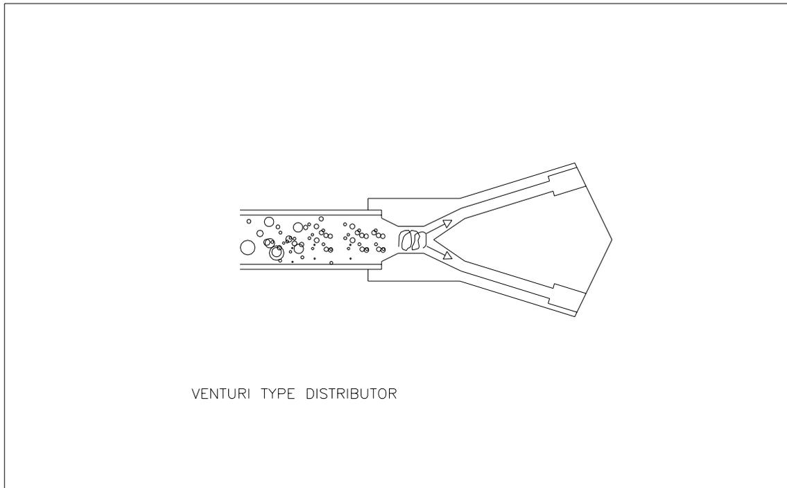
Venturi type distributors have a fixed tapered converging/diverging nozzle and are generally used on smaller equipment.
