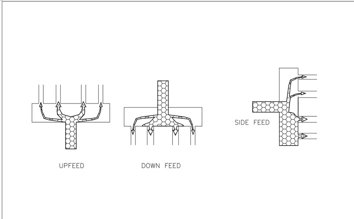
This diagram shows the effect of using a simple header in three different configurations.
